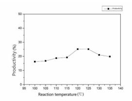
Fig. 6. The effect of reaction temperature on the productivity
